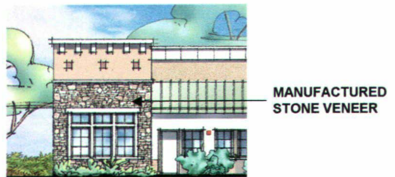
C. WALLS WITH MANUFACTURED STONE VENEER
